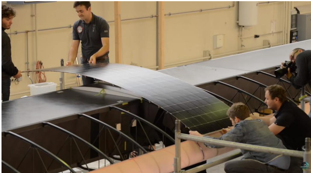
Figure 6. Wing construction of the Solar Impulse 2 aircraft.
