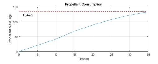
To overcome this and perform 2 takeoff and landing cycles, a larger amount of propellant would be needed.
