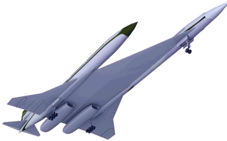
figure 6. Unusual Symmetry - Horizontal Tail
