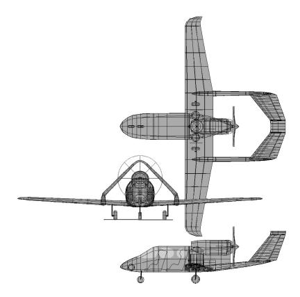
Since this was a small contract I did the analysis myself using RDS - aerodynamics, longitudinal stability, weights, and performance. It all checked out fine and the design requirements were met. Range and performance would be competitive with gasoline-powered propulsion systems, with only the current cost and availability of the "fuel" reducing the potential attractiveness of aircraft use for hydrogen fuel cells. Assuming, of course, that the fuel cell system numbers I was given were credible.
