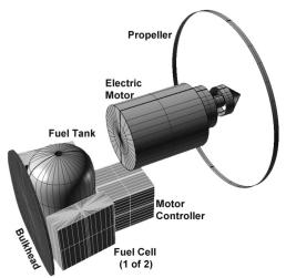
extreme pressure, so it needs to be a ball or a short capped cylinder. It also needs to be near the fuel cells themselves, flat battery-shaped boxes. The fuel cells should be fairly close to the motor and the almost-as-big motor controller. And the whole system together weighs over a thousand pounds. I decided to put it all together near the aircraft center of gravity, and close to the wing to make the structure lighter.
